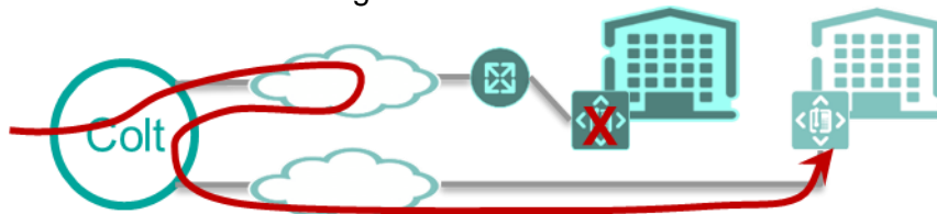
One active link to one active PBX, redirecting calls to another PBX in case of failure – Upon request
